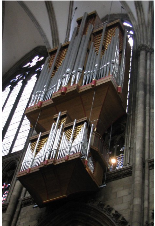
Illustration 3: The "Schwalbennestorgel" on the northern wall of the central nave (Klais, Bonn, 1998). Mechanical and (optional) electric action for remote control from the main organ console.
