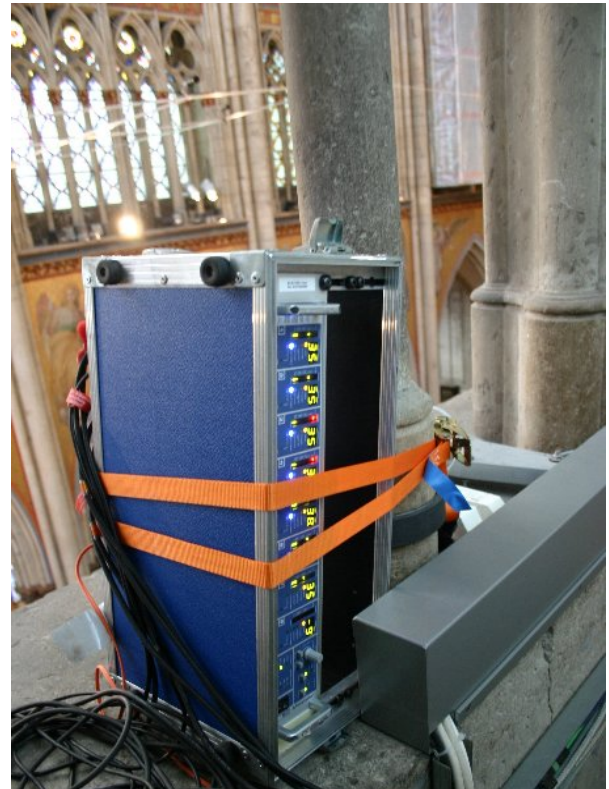
Illustration 7: One of the RME Micstasy remote controlled preamps, secured to a column on the Triforium. In the background, the Hamasaki frame can be seen.
