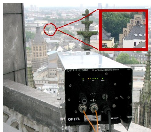
Illustration 4: The laser link seen from the intersection spire. The other end was located to the left of the staggered facade (the Overstolzenhaus, KHM library building).
