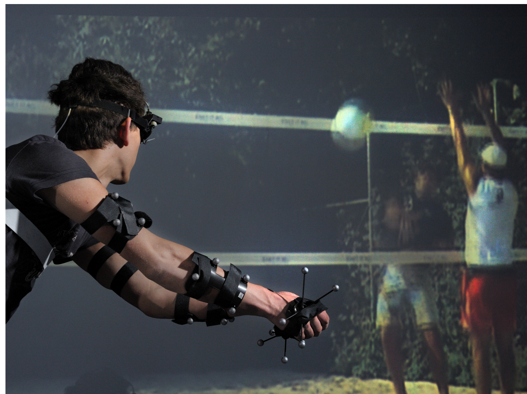
A typical experimental setup: determining decision accuracy and movement initiation time of expert beach volleyball players for different attack variations presented on a 3D projection screen. The participant is instrumented with Vicon infra-red reflective marks and an eye tracker.
