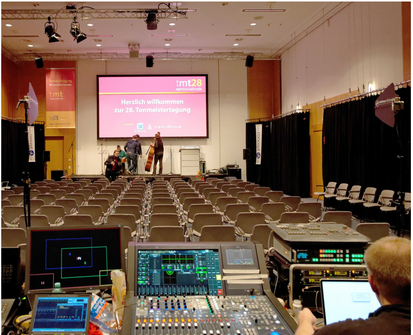
Fig. 7: The Auro 3D/Ambisonics room at tmt28, featuring two rings of eight and two ceiling speakers, two frontal subwoofers and one at the rear. All loudspeaker management tasks are performed by the console visible at the bottom. Acoustic curtains on three sides, with additional absorbers behind them.
