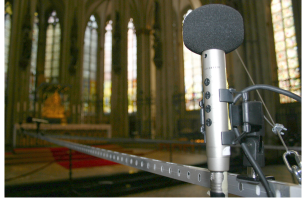
Illustration 10: Detail of the Hamasaki square, with one of the horizontal figures-of-eight (a Sennheiser MKH 800). The array was suspended in the central nave close to the apsis, at a height of around 20 metres.
