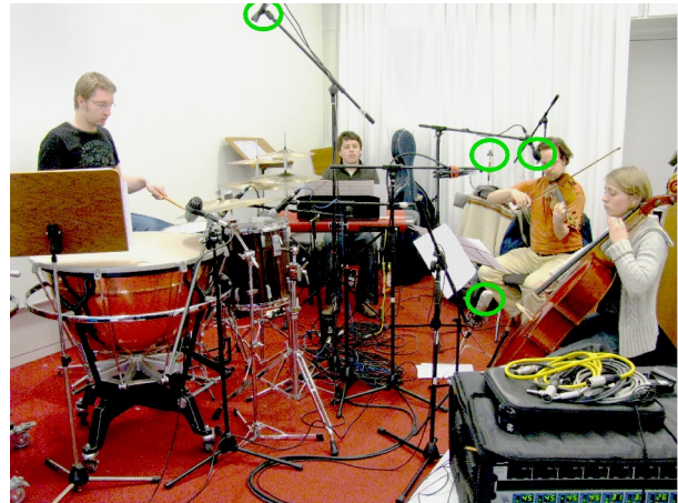
Illustration 1: Quartet session. Interesting mikes, top to bottom, left to right: coincident pair of AKG CK91s for drum set; Core Sound TetraMic as main microphone, offset towards the strings; AKG CK91 violin spot; BPM CR-95 cardioid cello spot
