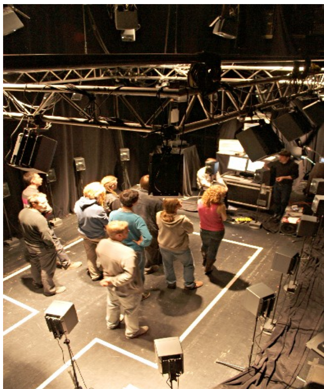
Illustration 4: ICSA playback setup, 40 Neumann KH-120 plus four KH 810.
